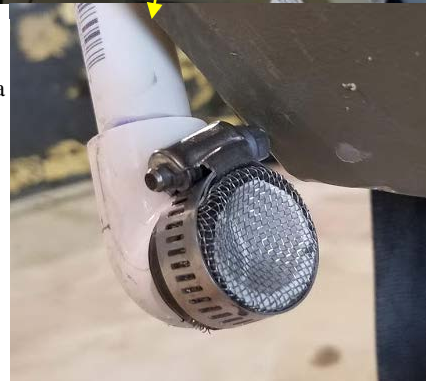
Figure 4.3: (Right) The PVC intake faces forward to push water into the system at high speeds. Wire mesh protects the pump and sensors from debris. We used PVC for its elasticity, and to prevent damage from impacts with logs or rocks.
